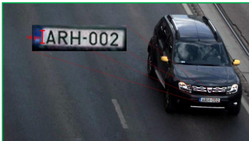
Figure 5: Optimal character size with optimal resolution for OCR: HD image. ✓
