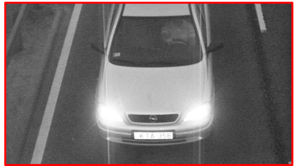
Figure 2: An overexposed image on which the license plate is barely visible. ✗
