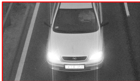
Figure 2: An overexposed image on which the license plate is barely visible. ✗
