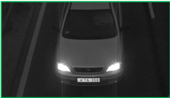
Figure 1: An image with good contrast. The characters on the license plate are clear. ✓
