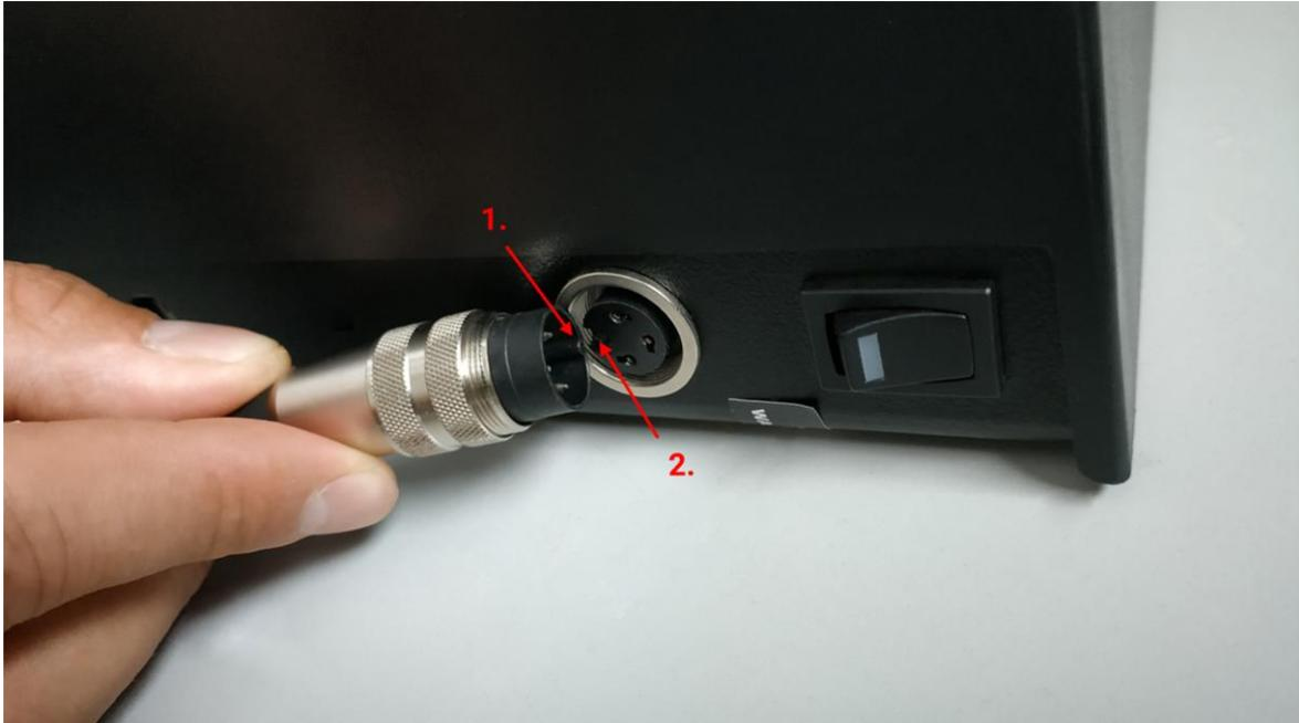
After connecting the power supply to the device, please screw on the plug to avoid accidental unplugging.
