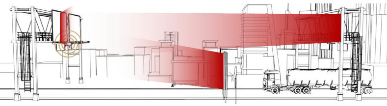
The camera (highlighted with golden circles) mounted beneath a highway road sign. The radar reflection from an approaching vehicle bounces off the sign, creating a second "virtual" image (ghost event) of the vehicle. This scenario can lead to unintended detections and potential inaccuracies.
