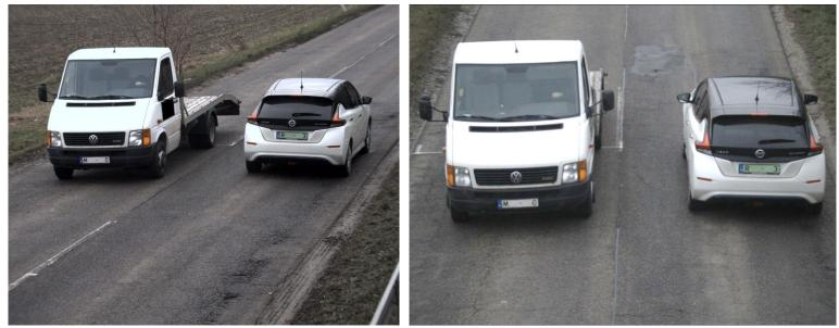
These images offer views captured by the cameras during the same event. On the left is CAM1 (pole), and on the right is CAM2 (gantry). It's important to note that while the camera effectively monitors only the Trigger Zone, the radar covers a more extensive road segment, both before and after the Trigger Zone. Therefore, the entire segment must be straight and unobstructed. The Trigger Zone should be around 1/3<sup>rd</sup> of the height of the image (or as close to the bottom as possible).
