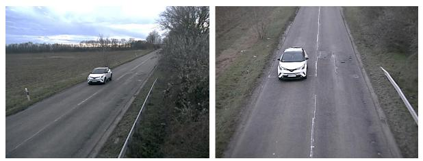
The Overview images are illustrating better, where the vehicles are located when they enter the Trigger Zone. The Trigger Zone is exactly at the optimal point, 30 meters (98 feet) away from the gantry.
