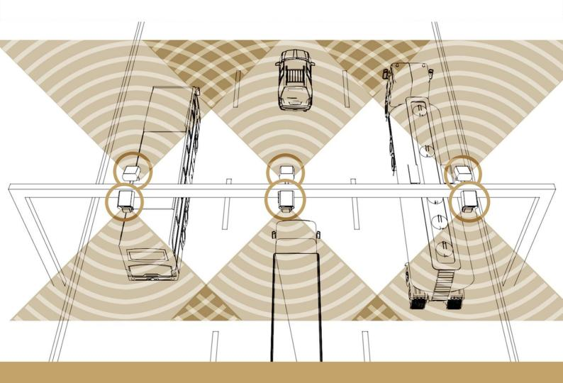
Installation Best Practices Guide for ANPR cameras equipped with multi-lane Radar.
