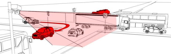
Note, how the radar might miss the incoming semi-truck, potentially hidden by the crossing traffic in the image below. The turning SUV enters the radar's view within the minimum tracking range, introducing the possibility of the radar failing to detect it.
