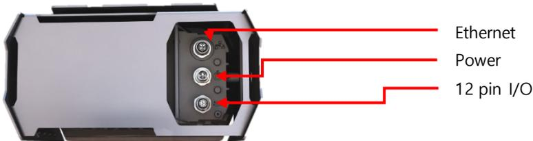
1.3 Make sure the connecting cable does not lead rainwater drops into the camera housing!
