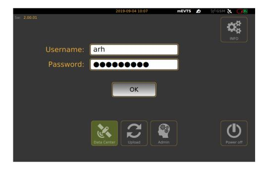
On the Login screen, select "Data Center" icon, type in Username and Password (click in to the empty field, touch-screen keyboard will pop-up, enter necessary characters, then press "Next" button), press OK, "Main" screen will appear.
