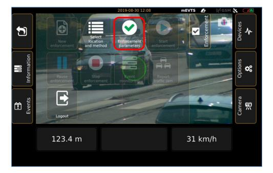
In the Enforcement parameters, optional control function can be chosen (selected functions appear green highlight), clicking on Next button to step on Speed limits. Description of each function will be discussed later.
