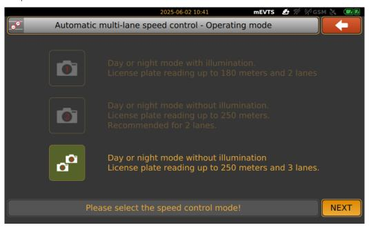
Choose the optimal layout based on camera placement:
