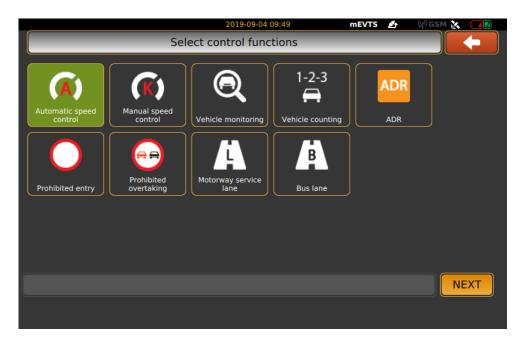
• Vehicle monitoring: creating an event of all passing vehicle with number plate, nationality, vehicle class, speed and distance.
