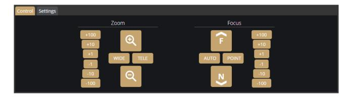
WIDE / TELE buttons: the lens can be adjusted to the end position using these buttons.
