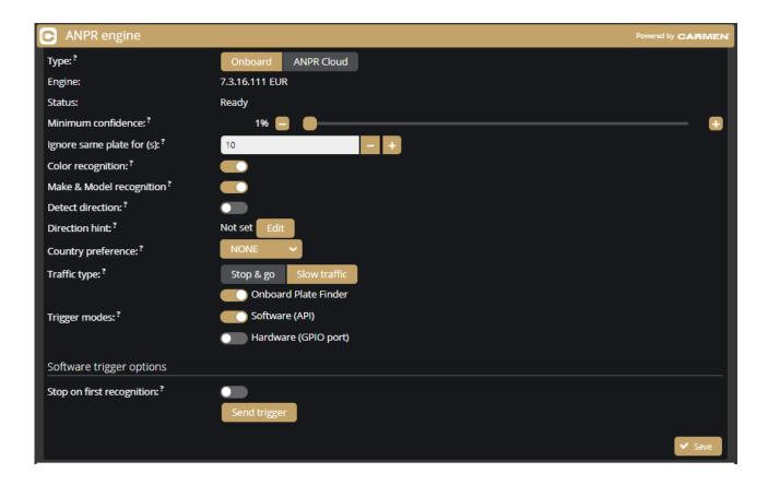
In the case of **Onboard ANPR**, you can adjust the primary functions of the ANPR engine. The parameters that can be set vary depending on the engine:
