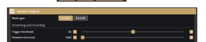
**Trigger threshold**: You can use it to define the sufficient level of motion in the image to trigger the motion engine. Further filtering can be done with the previously set sensitivity conditions to determine the degree of action intensity triggering recording. The **Motion graph** is the OSD belonging to the setting, which can provide visual assistance. See also **(Overlay)**.
