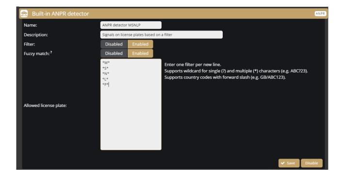
If you want to open a barrier when the above characters are detected, you have to enable the output port with the above detector in System / I/O menu at Trigger configuration section **{System / IO}**.
