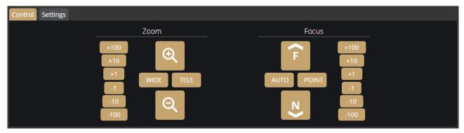
WIDE / TELE buttons: the lens can be adjusted to the end position using these buttons.
