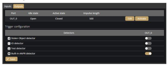
It can be selectable which detector signal should activate the output port of the camera at **Trigger** configuration section.
