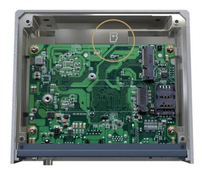
Step 4: Turn the MicroSD card upside down, and hold it with fingers at a 30 degree angle up from horizontal, and then insert and press it gently.
