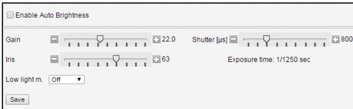
**Gain:** gain is the extent to which the sensor is amplified, resulting in brighter pixels. Note that high gain values result in noisy images.
