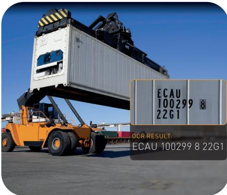
Shipping ports and logistics centers changed a lot in the past decades. Automatic Container Code Recognition (shortly ACCR) became almost a standard for building comprehensive databases – tracking container movement, automating and simplifying railway or harbor logistics, border control and container surveillance systems.
