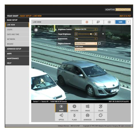
Brightness control will automatically monitor and control the exposure of the image, with license plate reading as a priority.
