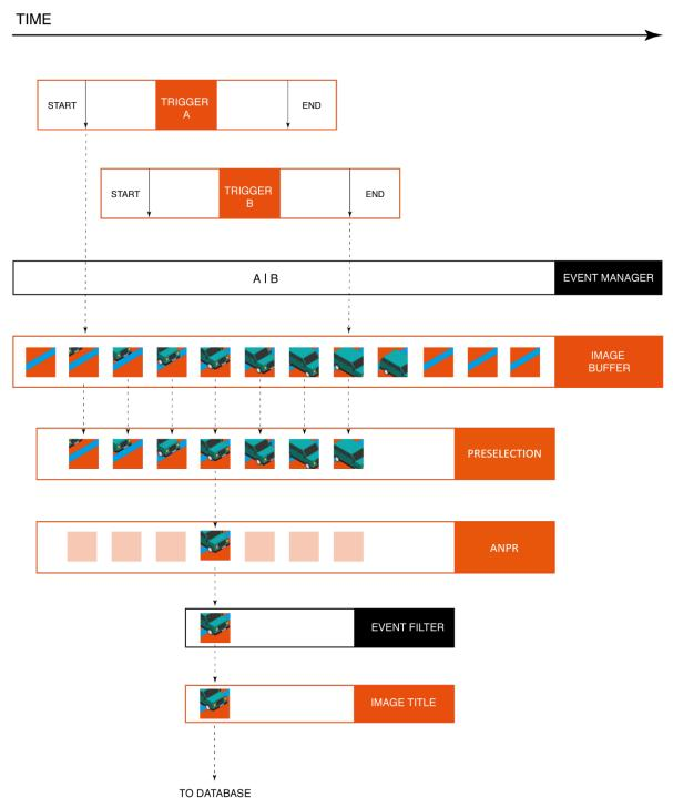
The above graphic is the schematic overview of trigger events being processed. License plate recognition operates as a multistage pipeline, taking a sequence of images of the same event as input, selecting one image of the vehicle (with the license plate in the best position), license plate and event data (textual form), and a license plate image as an output.
