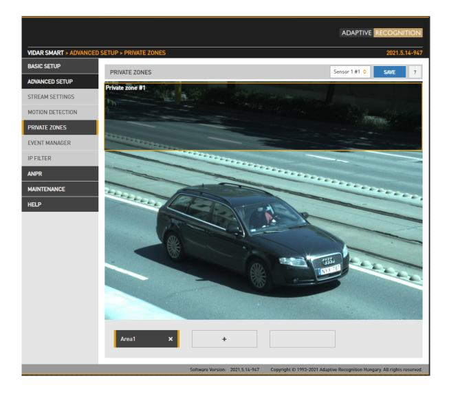
In certain circumstances it may be necessary to cover a part of the image, for instance, a parking place near the monitored lane, where the stationary vehicles should not be in the image, and their license plates should be excluded from processing, or when private property is displayed. These unwanted parts can be covered with a maximum of 3 rectangular zones using the Private zones tool.
