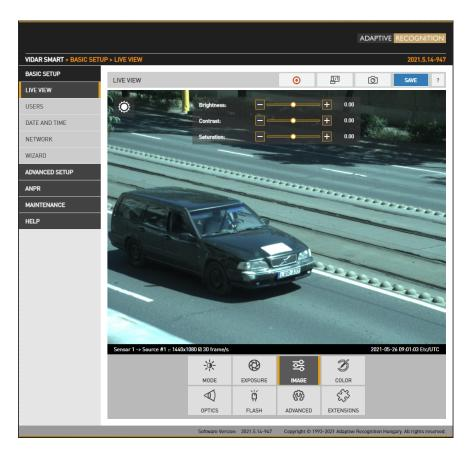
The basic post-processing settings are configured here: **Brightness:** Increase/decrease the brightness of the image
