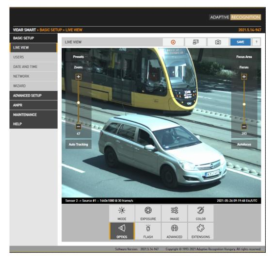
The live stream of the secondary sensor is shown in the box below (picture in picture). By clicking the live stream box, the main view switches to the secondary sensor, and all settings (Brightness control, Color, Optics etc.) will be applied to the secondary sensor.
