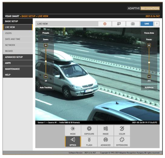
Models equipped with motorized lenses will show this menu item. Both lenses can be adjusted individually by switching between the two sensors in the Live view menu. Use the left slider (Zoom) to change the field of view from wide angle (0) to telephoto (100). Use the right slider (Focus) to manually adjust focus from near too far.
