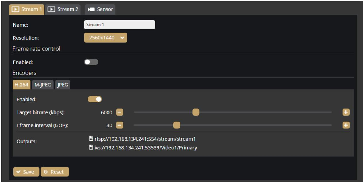
On this interface the settings (name, resolution, frame rate etc.) of the **Stream 1** and **Stream 2** can be performed separately. The **H.264** and the **MJPEG** versions of the streams can be adjusted separately as well as the quality of the thumbnail images also can be defined.
