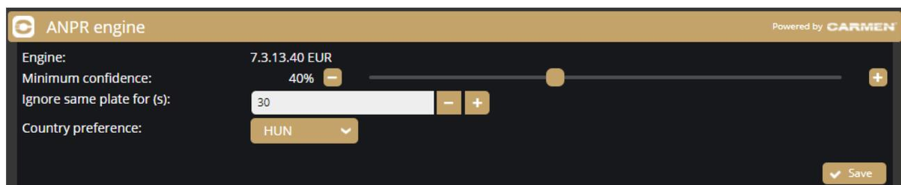
A mask can be created on the image, after which license plates will be detected only in the selected area. It is recommended to limit the searching area as much as possible, thus facilitating recognition. The ANPR engine recognizes the number plates in the image, but in order for the engine to work properly, the area around the number plate must be visible (front or rear of the vehicle).
