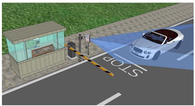
Try to adjust the direction of the camera so that the number plates are horizontal in the picture!
