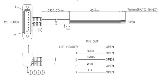
PIN4: IO\_I\_N (black) PIN5: IO\_I\_P (brown) PIN6: IO\_O\_A (white) PIN7: IO\_O\_B (blue)
