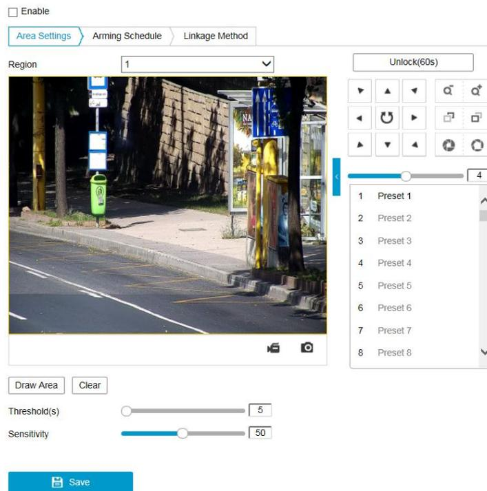
Figure 5-26 Configuring Region Exiting Detection
