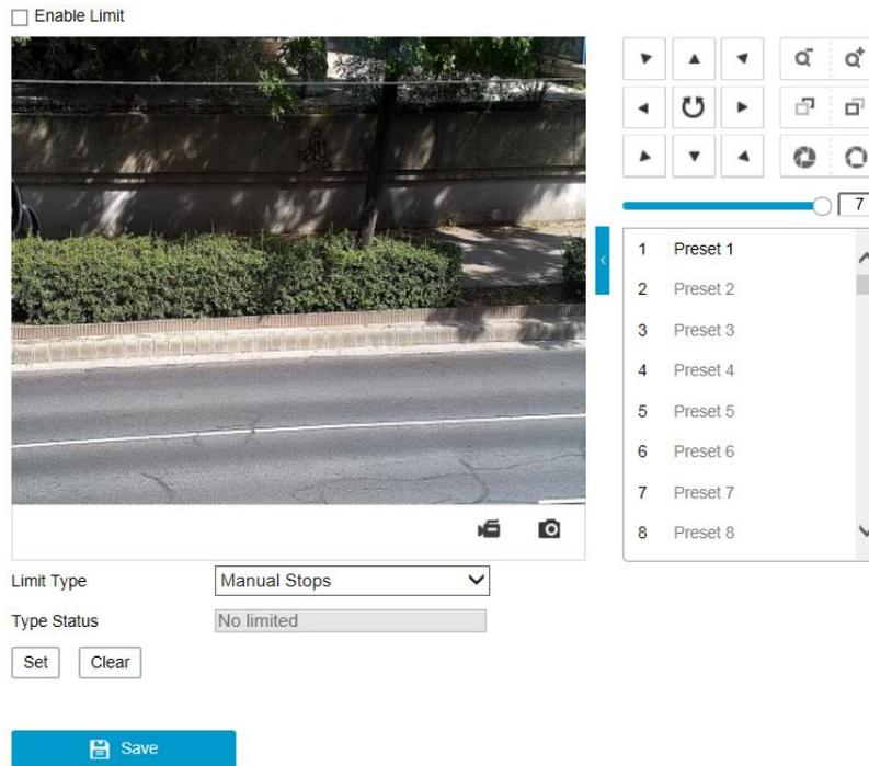
Figure 5-29 Configure the PTZ Limit
