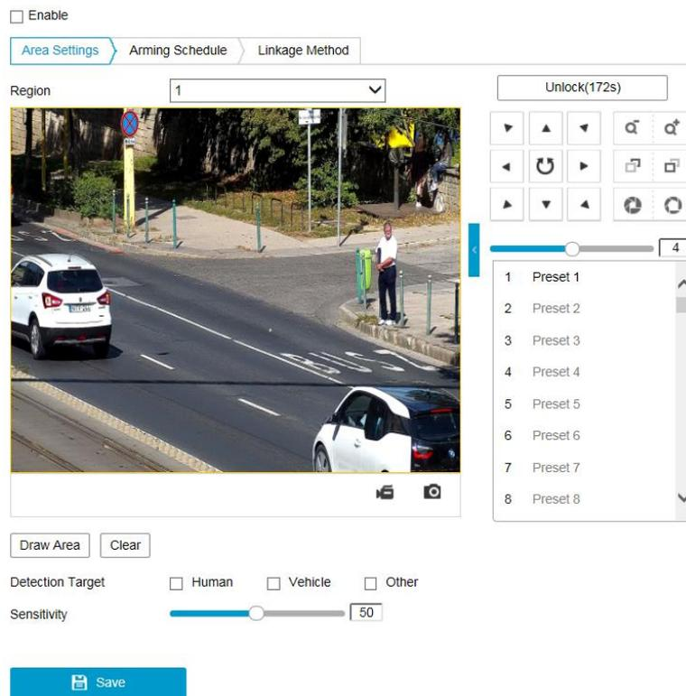
Figure 5-25 Configuring Region Exiting Detection
