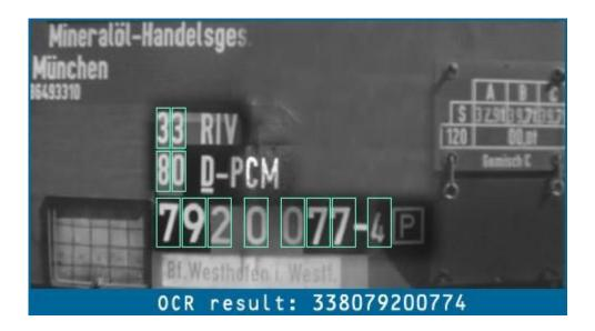
**CARMEN<sup>®</sup> OCR** is an optical character code recognition software of **ARH Inc**, designed for codes in the cargo and transportation sector. It provides an easy-to-program Application Programming Interface (API) for software developers.
