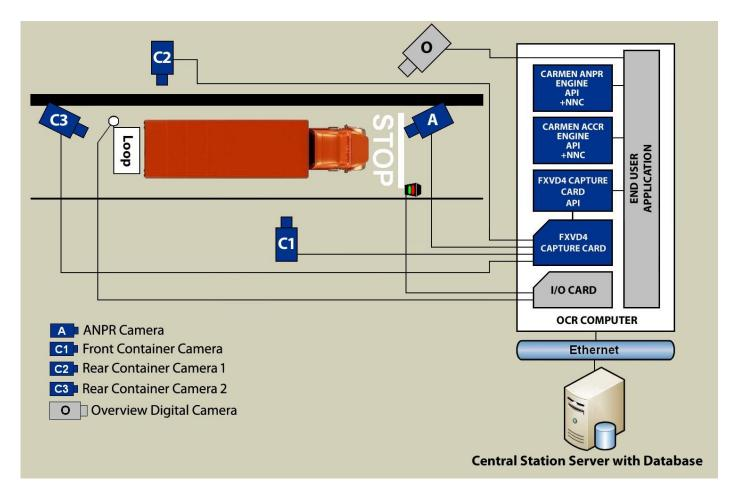
**NOTE**: The FXVD4 capture card and API is only needed in case of analog CCTV cameras.
