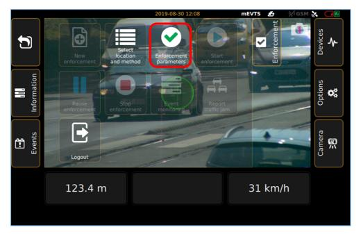
In the "Enforcement parameters", optional control function can be chosen (selected functions appear green highlight), clicking on "Next" button to step on "Speed limits". Description of each functions will be discussed later.
