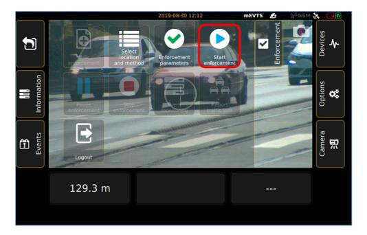
By click on "Start enforcement" icon, screen will guide you to the "Check of location parameters" to verify all values, if It is correct, press "Accept" and start enforcement. If need more adjustment or correction during the setup, you can clear all setup until now and go back to the main window.
