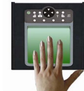
The fingers are in the middle of the platen in vertical position.
