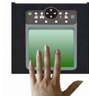
The fingers are too near to the side of the platen.
